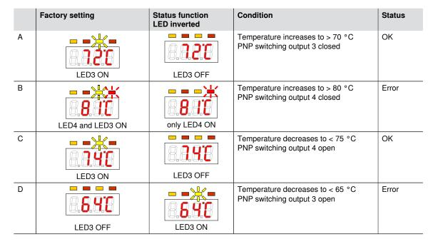
Here, you can reverse the LED status function for a contact: the LED is illuminated if the contact is open, i.e. below the minimum temperature, and the "Error" status is indicated again if the LED is illuminated. The recording of events particularly depends on the lighting up of the LED (see chapter "Diagnosis possibilities", 4.9).
