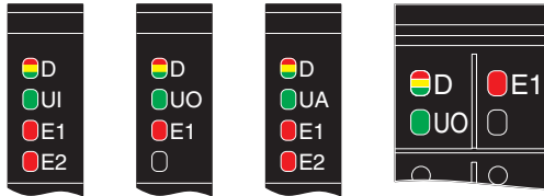
Fig. 2-3 D and E LEDs on the power connectors of the I/O modules (examples)
